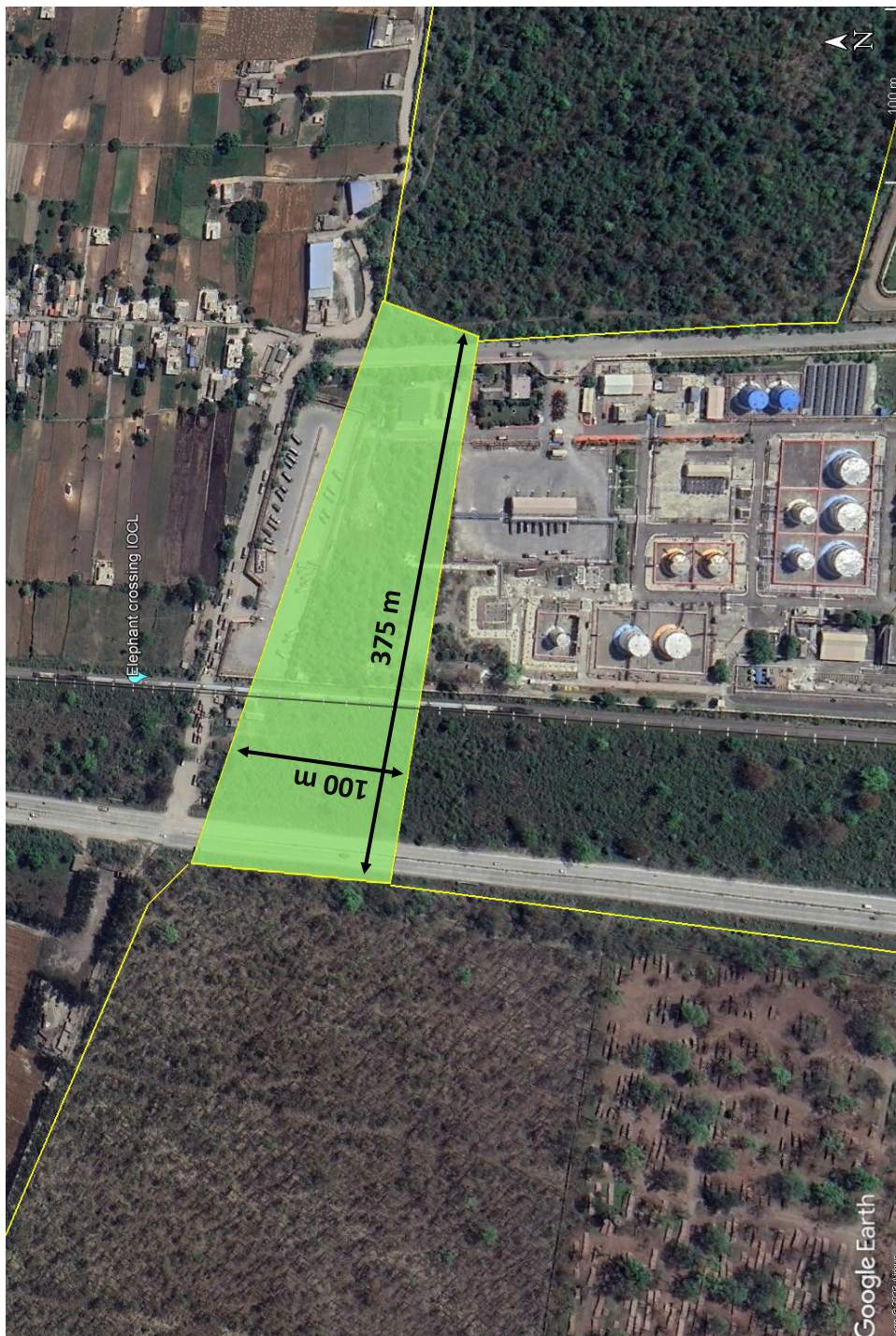
Figure 7: Suggested location of the wildlife overpass over the NH 109, railway track and IOCL compound (green polygon) and fencing (yellow lines) funnel wildlife movement towards the overpass.
