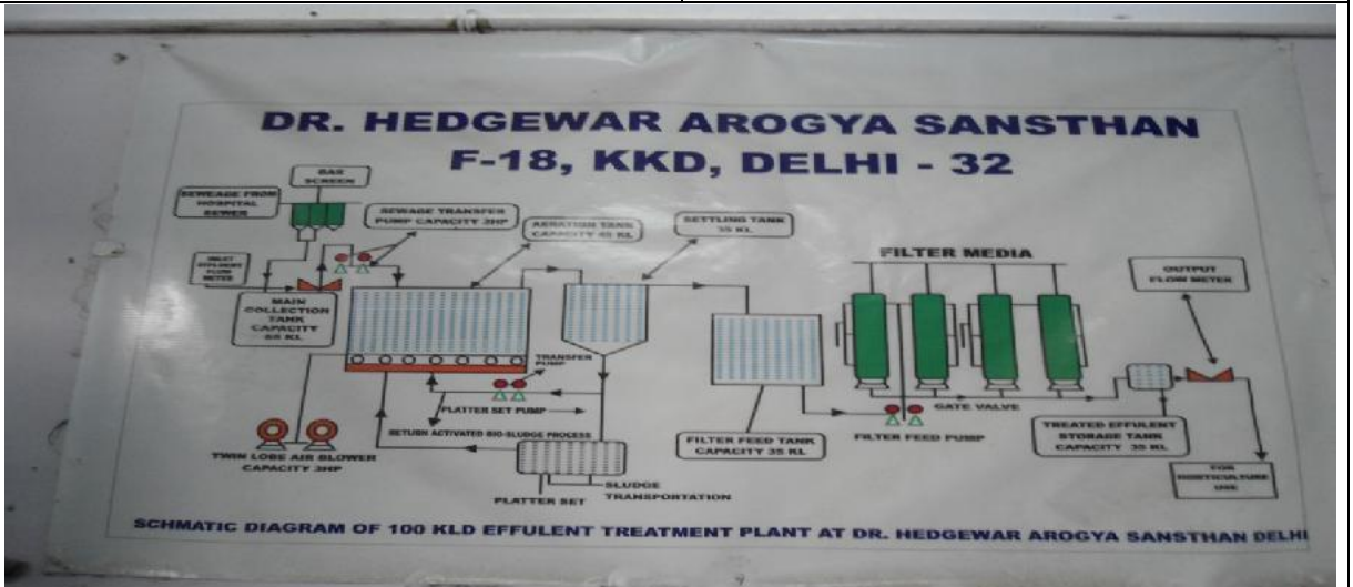
Waste Water Treatment Process Flow Chart
