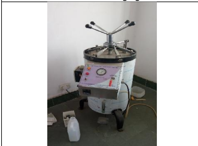
Pre-treatment of BMW by autoclave
