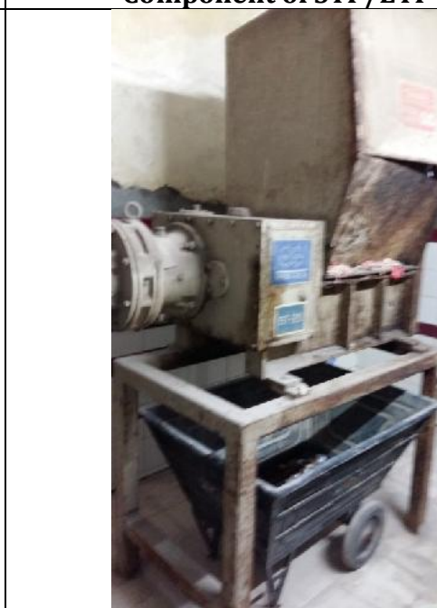
On-site autoclave and shredder installed by the hospital
