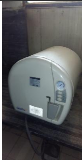
Pre-treatment of waste using Autoclave and Dry Heat Sterilisation
