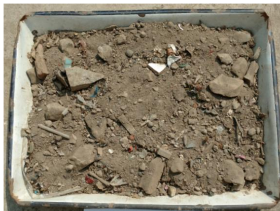
Fig 24:-view of final material selected for embankment construction.
