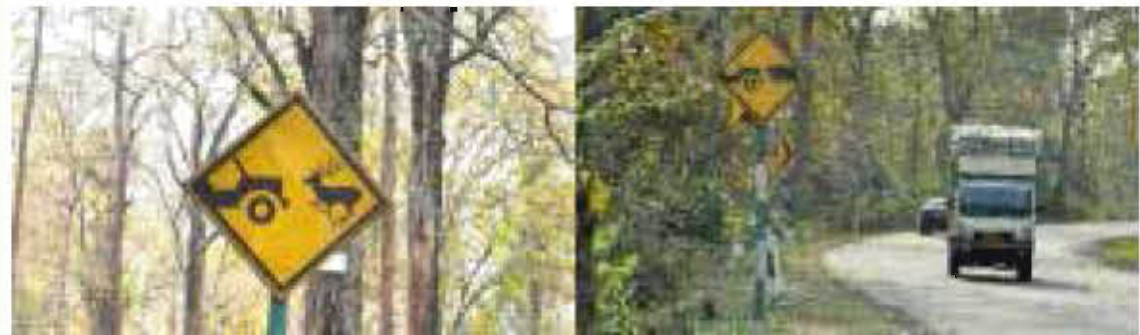
Figure 10.2. Simple caution signs to alert drivers of animal-movement areas to reduce animal vehicle collisions (AVCs) in NH 6 and 7 in India.
