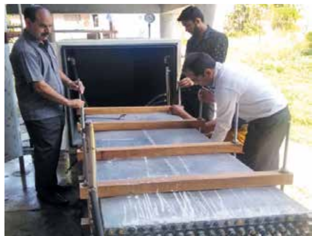
Fabrication and installation of a 'Solar Vacuum Wood Dryer capable of thermal energy storage
